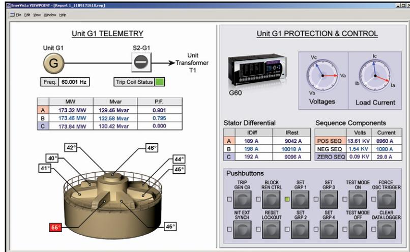
The UR is the single point for protection, control, metering, and monitoring in one integrated device that can easily be connected directly into DCS or SCADA monitoring and control systems like Viewpoint Monitoring as shown.
