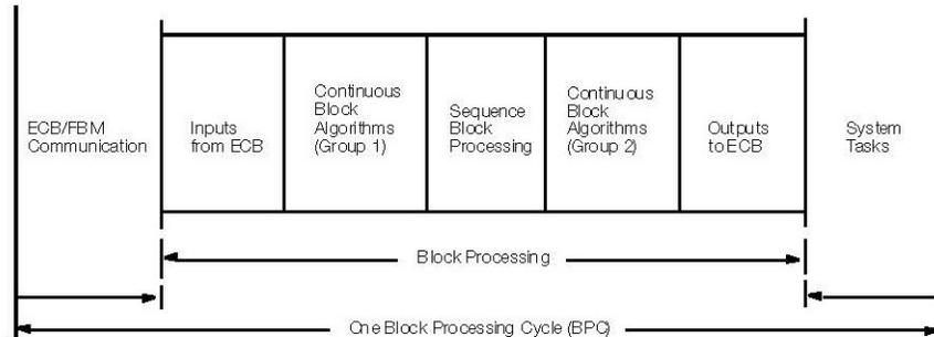
At the beginning of block processing, I/O data is read from each Fieldbus Module, for both input and output channels. Data is read at the ECB scan period specified for that module. However, data cannot be read faster than the BPC. At the end of block processing, process outputs are written to each of the Fieldbus Modules.
