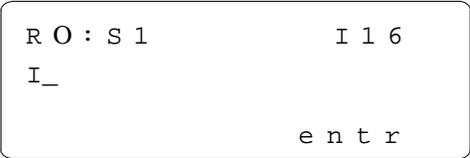
Specify the I/O references to be used by the module. For most applications, you can simply have the BIU/Field Processor assign the next available references in that memory type.
