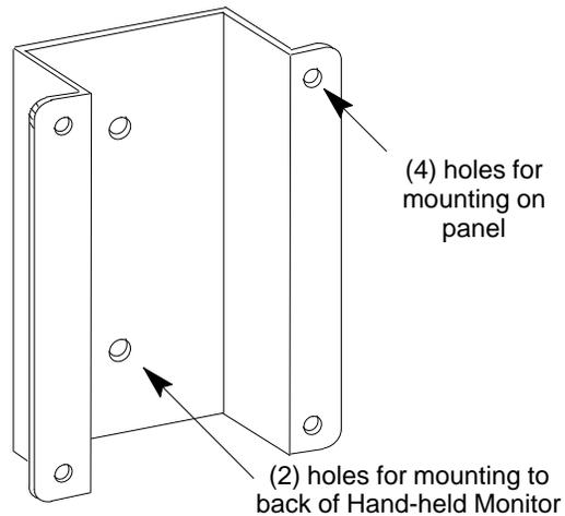
4. Using appropriate hardware (not provided), mount the HHM and bracket in the cutout.
