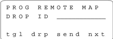
3. Press the F3 (send) key to download these selections to the Remote I/O Scanner.
