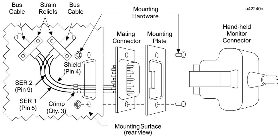
When making bus connections, the maximum exposed length of bare wires should be two inches. For added protection, each shield drain wire should be insulated with spaghetti tubing to prevent the Shield In and Shield Out wires from touching each other.
