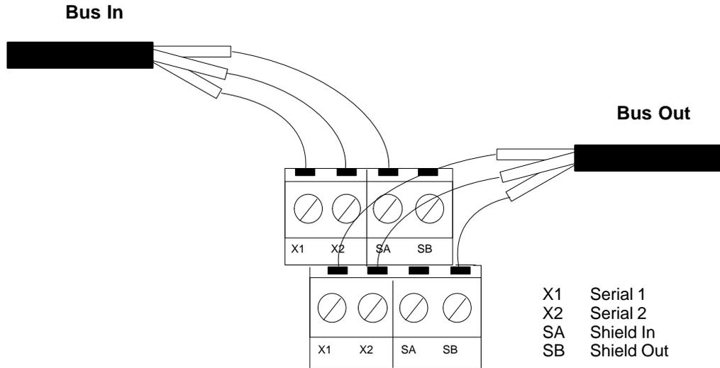
As with other devices, if the HHM Connector is at either end of its bus, install an appropriate terminating resistor across the Serial 1 and Serial 2 terminals. The *Genius I/O System and Communications User's Manual* lists appropriate terminating resistors for each recommended bus cable type.
