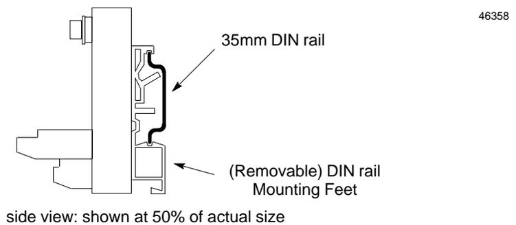
Alternatively, it can be installed directly on a panel using screws through its mounting ears. The DIN rail feet on the back of the unit are removed when the unit is panel-mounted.
