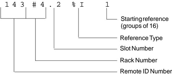
The Series 90-70 I/O reference for the circuit is one less than the sum of the two numbers on the righthand side of the HHM screen. For example:
