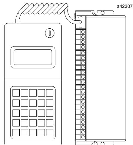
2. Turn the Hand-held Monitor on. After the HHM completes its powerup sequence, the Home menu appears. The Hand-held Monitor's Change Block Configuration option must be enabled to complete the instructions in this section. For a new device, the HHM's Change Block ID and Change Block Baud options must also be enabled.
