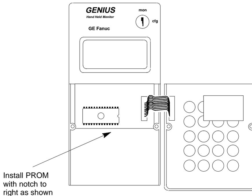
6. Remove the old PROM. If you don't have a PROM extraction tool, a small screwdriver can be used instead, carefully working from side to side.
