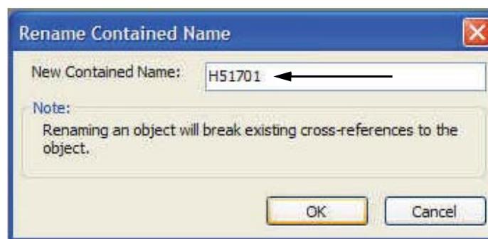
Figure 4-27. Renaming an ECB201 for an LB 3102 (HART) Module's HART Device in IEE (Example)
