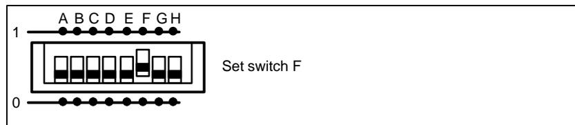
Fig. 4.27 Function switch on the rear of the external MO drive
