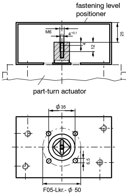
Figure 3-11 Attachment of part-turn actuator, mounting console (scope of delivery actuator manufacturer), dimensions
