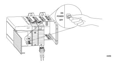
2. Set the mode switch on the controller to REM.
